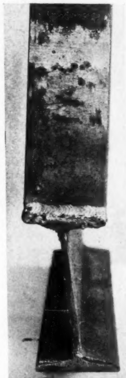
FIG. 3. END VIEW OF STATIC TEST PIECE SHOWING FAILURE IN BASE
